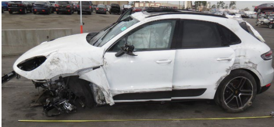
Figure 7. Left plane damage, 2021 Porsche
