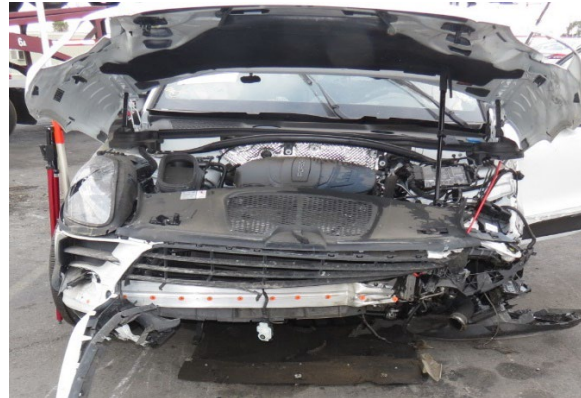
Figure 8. Front plane damage, 2021 Porsche Macan
