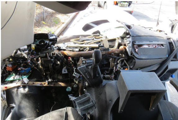
Figure 5. Severe intrusion damage of ambulance's instrument panel (image taken from center of cab)
