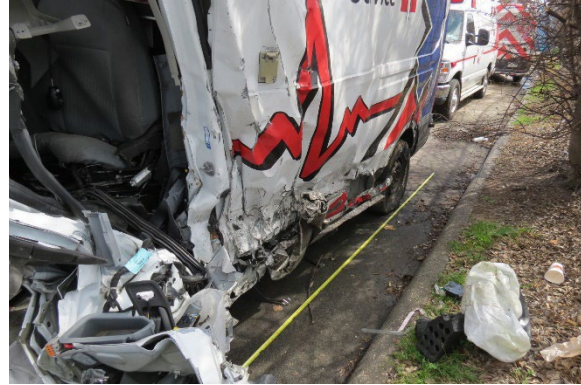
Figure 4. Left sill damage
