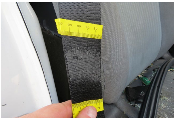
Figure 7. Load mark on right passenger's belt webbing
