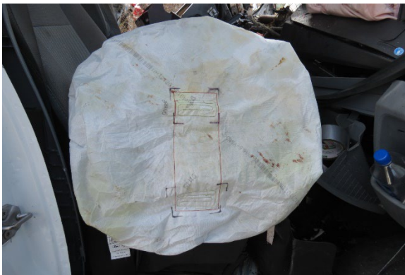
Figure 9. Discolored face of driver's frontal air bag
