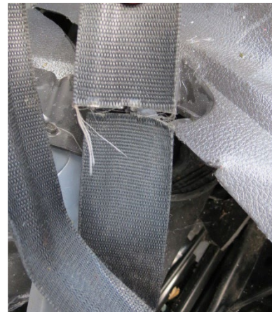
Figure 6. Driver's lap belt cut by rescue personnel
