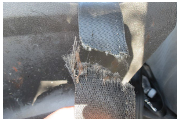
Figure 8. Driver's seat belt webbing cut near D-ring
