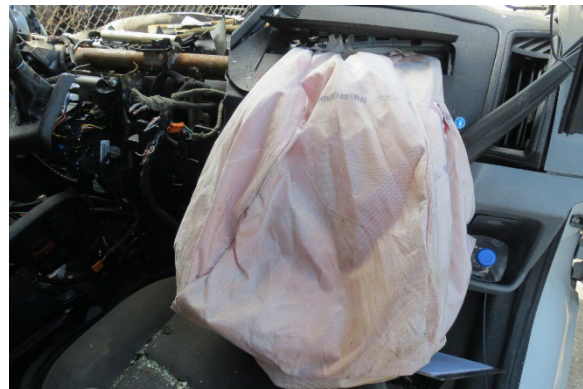
Figure 10. Deployed passenger's frontal air bag
