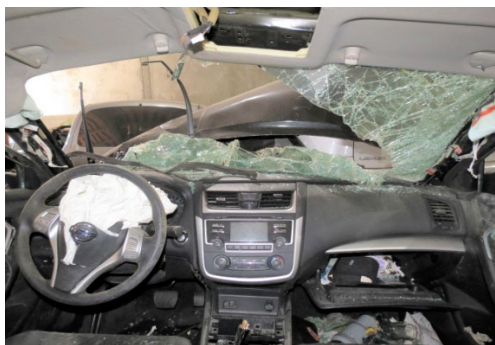
Figure 7. Front row damage, 2017 Nissan Altima
