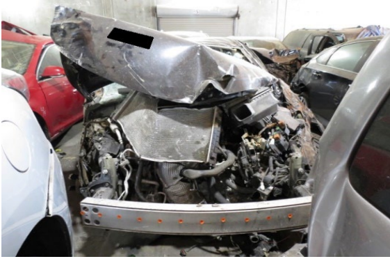
Figure 4. Front plane damage, 2017 Nissan Altima
