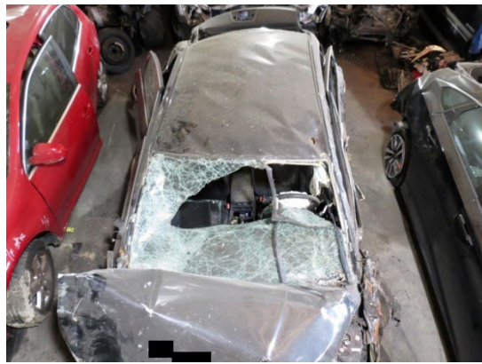
Figure 6. Top plane damage, 2017 Nissan Altima
