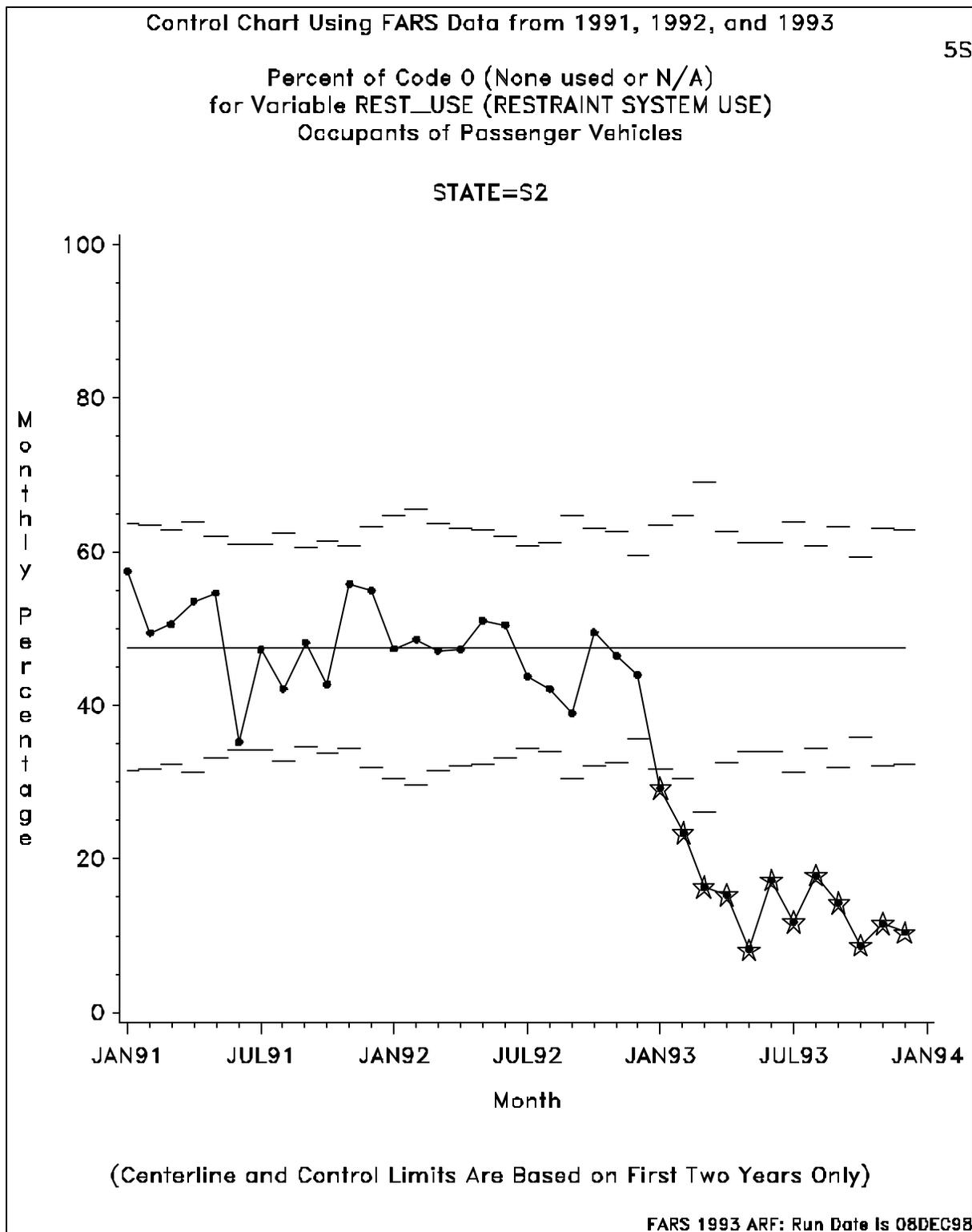
Figure 2. A Control Chart Out of Statistical Control.
