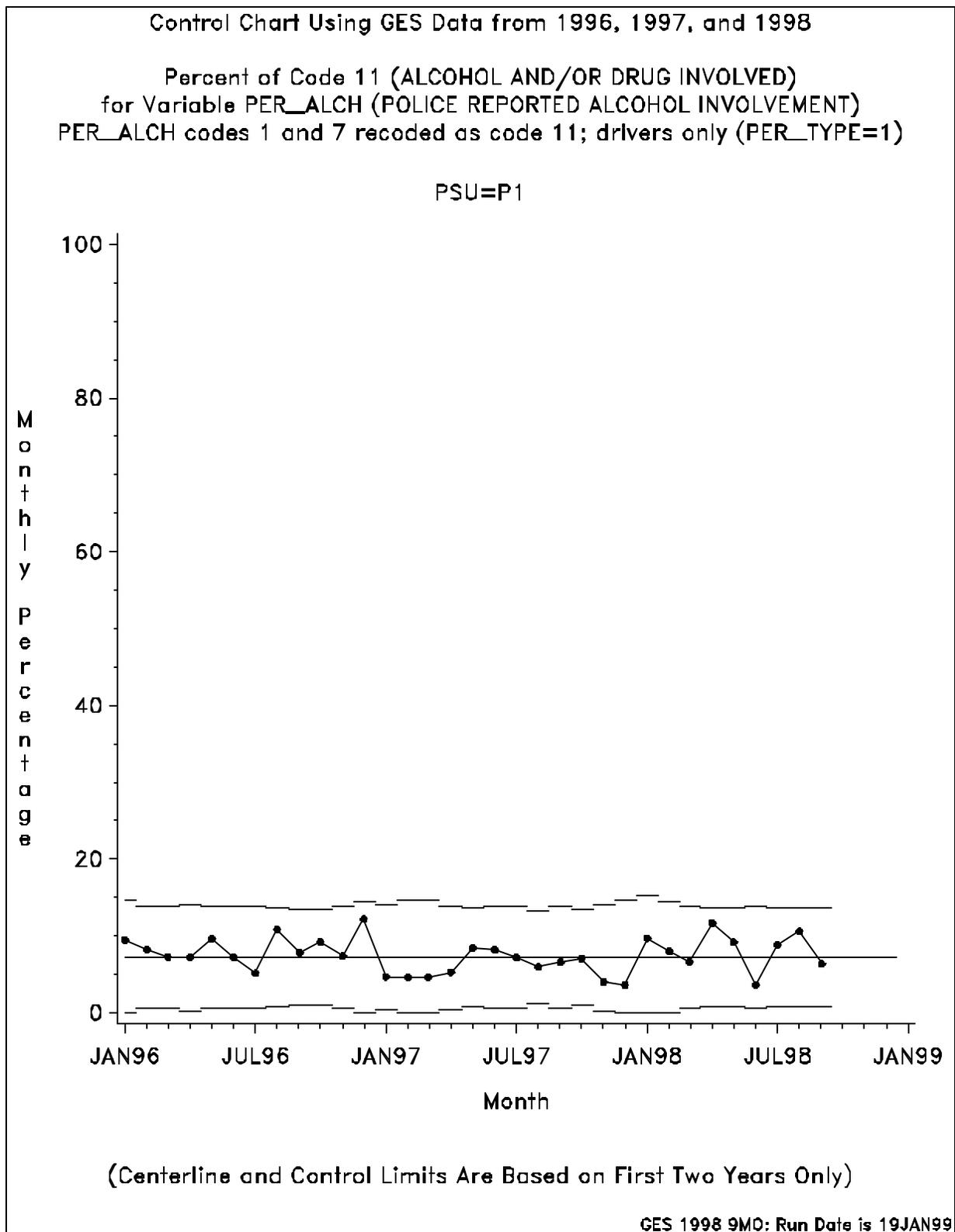
Figure 1. An Example of a Control Chart in Statistical Control.
