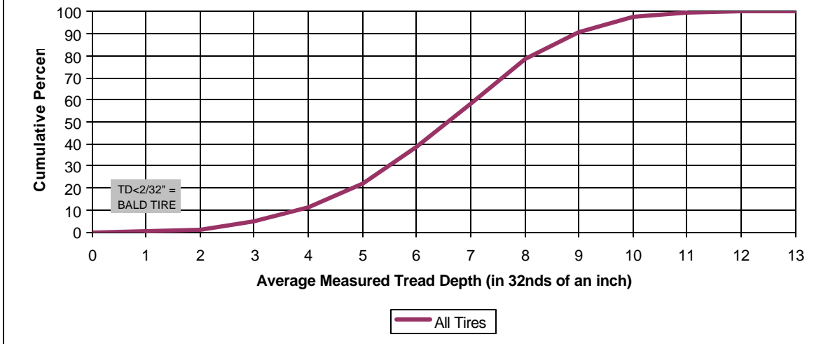
Figure 4 Cumulative Percent of the Average Measured Tread Depth for Each Vehicle
