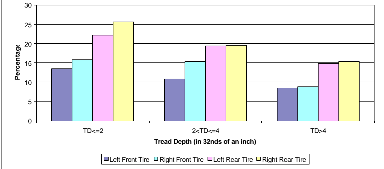
Figure 9 For the Given Ranges of Tread Depth, the Percentage of Tires Underinflated by 8psi or More (by Tire)
