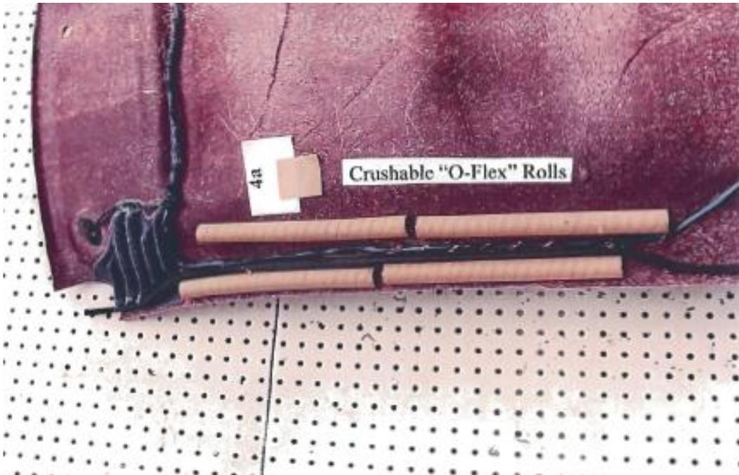
Figure 1-4: Crushable O-Flex Rolls<sup>18</sup>
