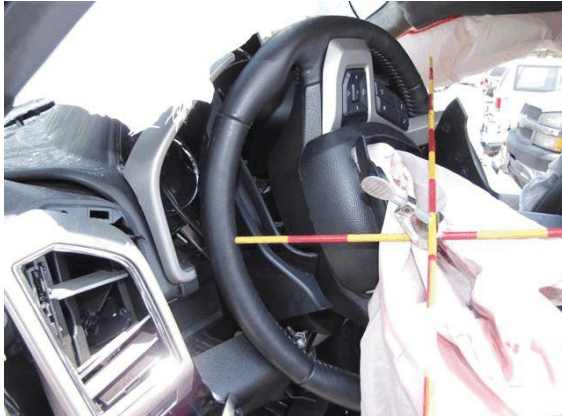
Figure 8. Bent steering wheel rim, driver contact point, the 2017 Ford F-250
