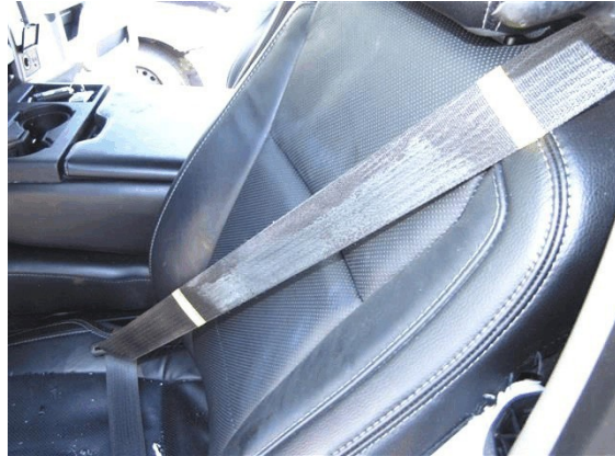
Figure 9. Scuffed and stretched seat belt, driver loading point, the 2017 Ford F-250
