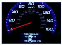
If Option 11.3, "Tire specific psi" was chosen, the data collector recorded, in the spaces provided on the form, the individual psi that were seen on the vehicle's TPMS display.
