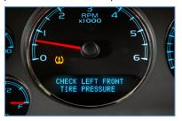
**11.3:** Tire Specific psi – Always provides the psi for each of the tires. The psi is provided not only when the tires are under or over inflated, but also when they are properly inflated.
