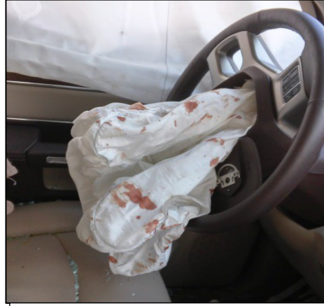
Figure 14: Deployed driver frontal air bag in the RAM. Image supplied by the driver.
