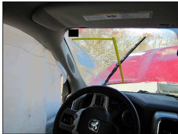
Figure 11: Fracture pattern to the windshield glazing resultant from driver contact during the crash.
