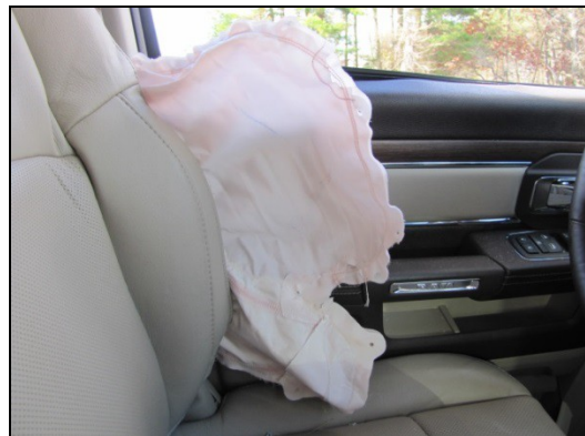
Figure 15: Deployed driver's seat-mounted side impact air bag in the 2014 RAM 1500.
