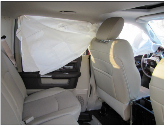
Figure 10: View of the RAM's interior and the left B-pillar engaged against the driver's seat.
