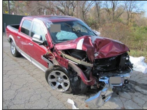
Figure 7: Front right oblique view of the RAM and the damage associative to Event 3.
