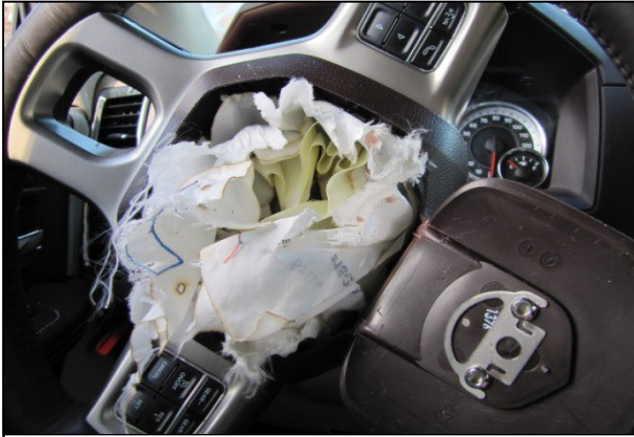
Figure 13: Driver frontal air bag fabric cut from the module in the RAM at the time of the SCI inspection.
