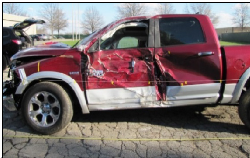
Figure 8: Left plane view of the RAM and the Event 4 deformation pattern from the third tree impact.
