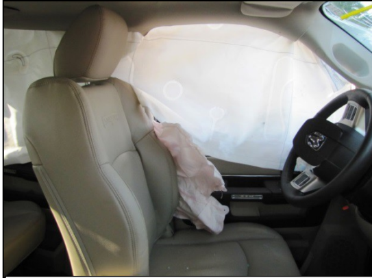
Figure 17: Left IC air bag and deployed driver's seat-mounted air bag in the 2014 RAM 1500.
