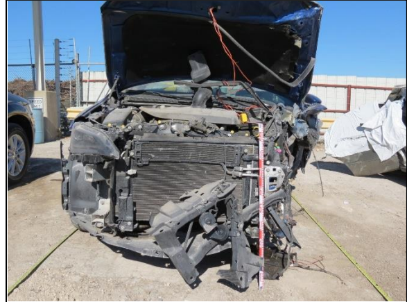
Figure 3: Damage to the front plane of the Chrysler from impact with the front plane of the Ford
