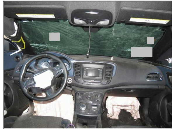
Figure 6: Overview of occupant contact of left A- pillar (yellow tape), steering wheel, and instrument panel
