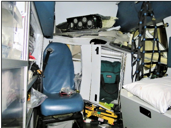
Figure 12: Forward-facing view of the patient compartment interior and crash-related damage.
