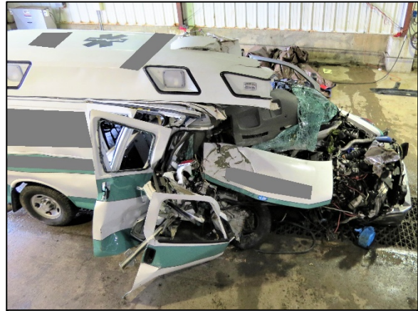
Figure 10: Right overhead perspective view of the ambulance and the magnitude of the damage extent.
