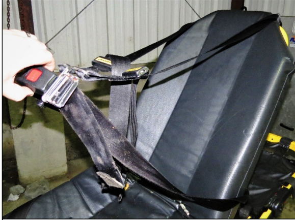
Figure 17: Shoulder harness straps of the Stryker cot after being buckled together by the SCI investigator.
