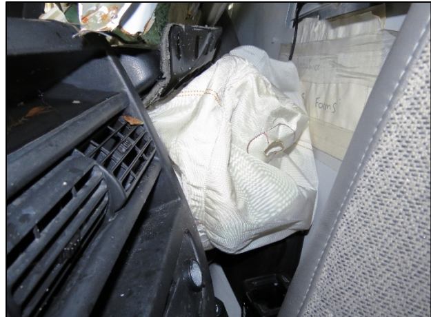
Figure 15: View of the deployed front right passenger's air bag at the time of the SCI inspection.
