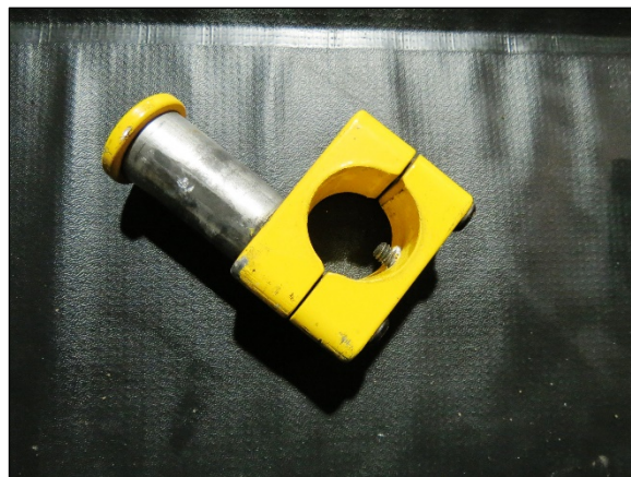
Figure 19: Separated locking pin found loose in the patient compartment during the SCI vehicle inspection.
