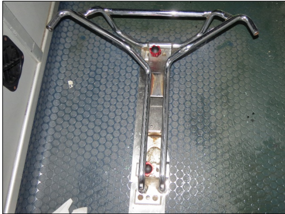
Figure 20: Antler bracket of the cot fastening system mounted in the Chevrolet ambulance.
