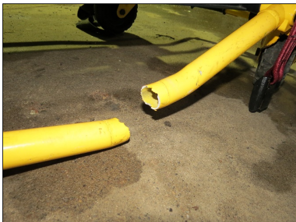
Figure 18: View of the sheared lower right frame rail of the wheeled ambulance cot.
