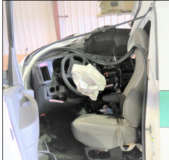
Figure 11: Crossing view of the ambulance cab and the severe interior damage/intrusion
