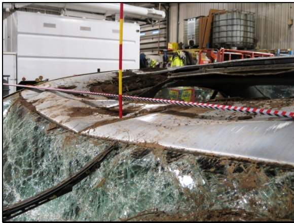
Figure 12: Vertical deformation to the Volkswagen's windshield header associative to the rollover event.
