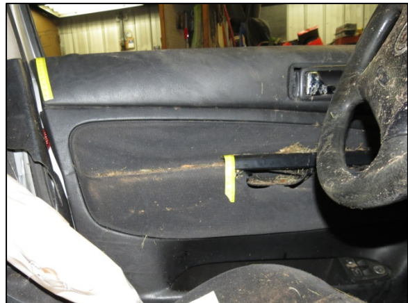
Figure 15: View of the Volkswagen's left front door with contact evidence from the driver to the armrest and rear upper quadrant.
