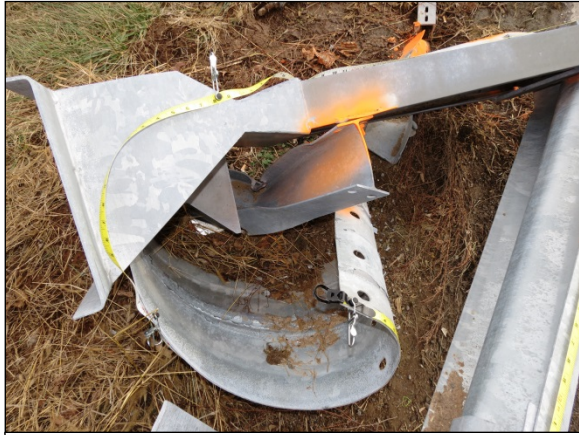
Figure 7: View of the impact head and extruded rail from an overhead perspective.
