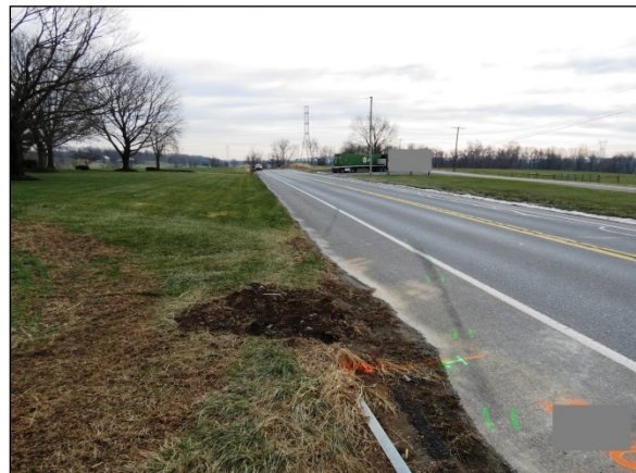
Figure 4: South-facing view of the Volkswagen's yawing tire marks and roadside departure from beyond the location of the end terminal impact.
