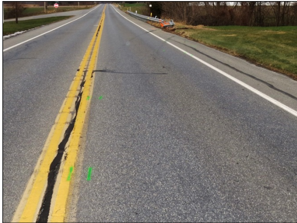
Figure 3: North-facing view of the tire marks from the Volkswagen's left rear, left front, and right front tires that evidenced the vehicle's clockwise yaw and control loss.
