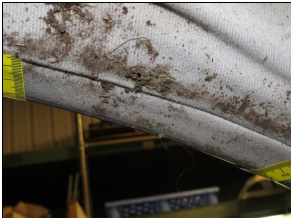
Figure 14: Image depicting strands of hair captured in the weather stripping near the left roof side rail from contact by the driver's head during her ejection.
