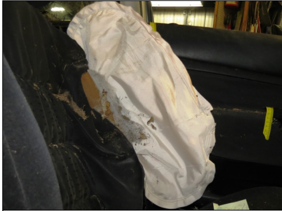
Figure 17: Driver's deployed seat-mounted side impact air bag in the Volkswagen at the time of the SCI vehicle inspection, with post-crash dirt/debris.
