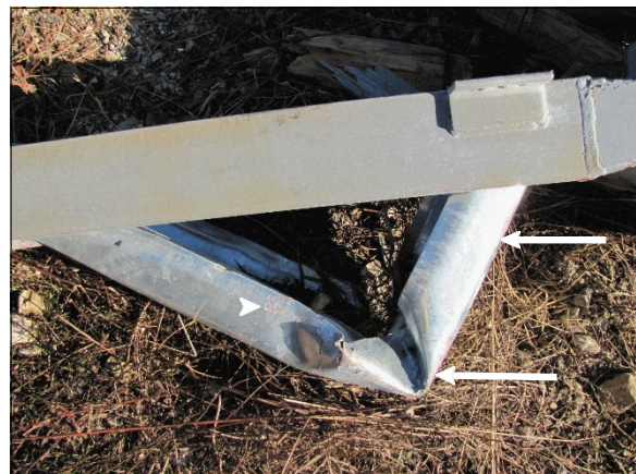
Figure 12: The kink within the ET-2000; arrows show red paint from contact with Toyota's left rear door
