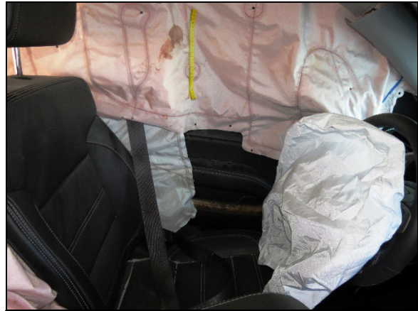
Figure 14: View of the deployed driver's frontal, driver's seat-mounted side-impact, left IC, and center seat-mounted air bags within the GMC.
