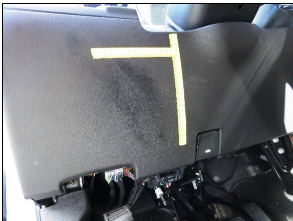
Figure 11: Driver left knee contact to the left lower instrument panel.
