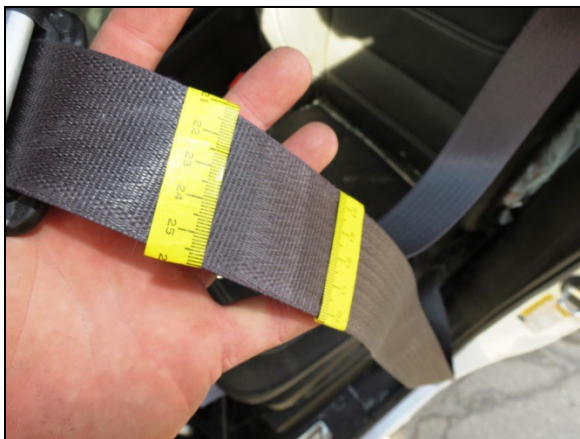
Figure 13: Frictional abrasion on the GMC’s lap belt webbing from driver loading against the latch plate.
