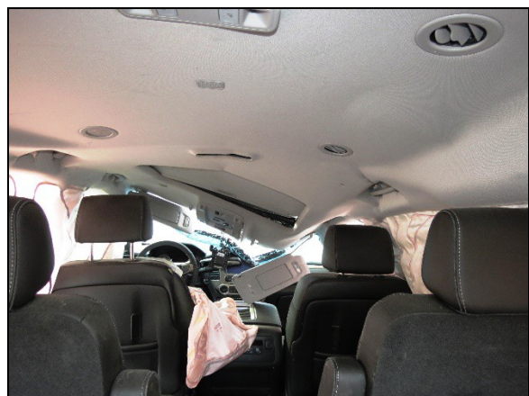
Figure 12: Forward-facing view of the GMC’s interior depicting the significant vertical intrusion of the roof.
