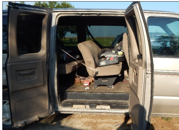
Figure 3: Police photo showing step in right rear door frame
