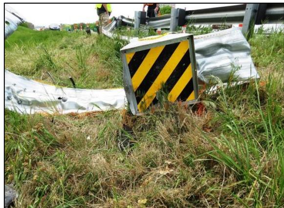
**Figure 9:** Image depicting the impact-face of the end terminal looking to the west.
