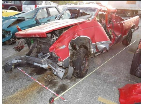
**Figure 1: Left front oblique view depicting the deformation of the 1991 GMC Sonoma.**
