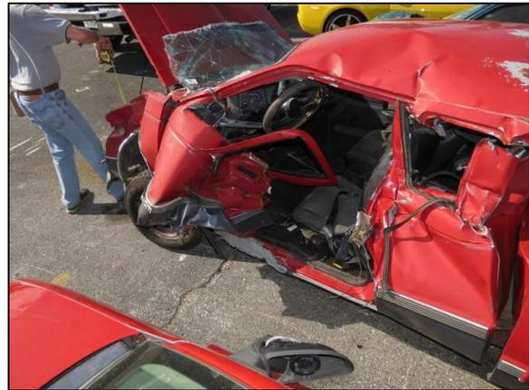
**Figure 14: Left view of the GMC depicting the impact damage and intrusion at its left door.**
