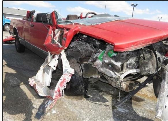
**Figure 12: Front right oblique view of the GMC depicting the impact damage.**
