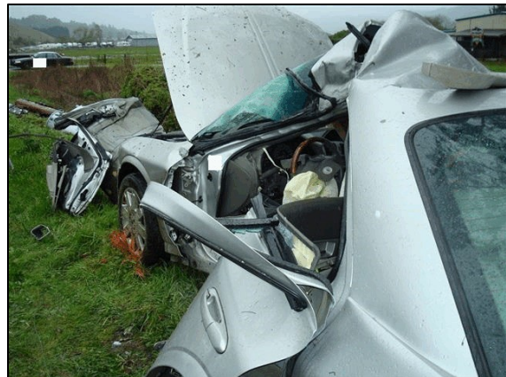
Figure 6. Direct damage to left roof, 2004 Lincoln LS (police photo)
