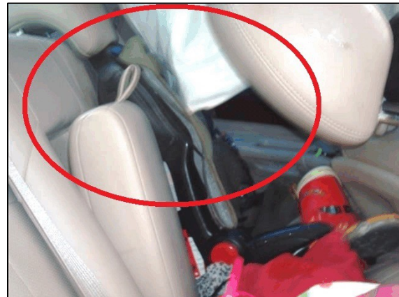
Figure 8. Deployed left IC air bag and CRS installed in second row left position, 2004 Lincoln LS (police photo)
