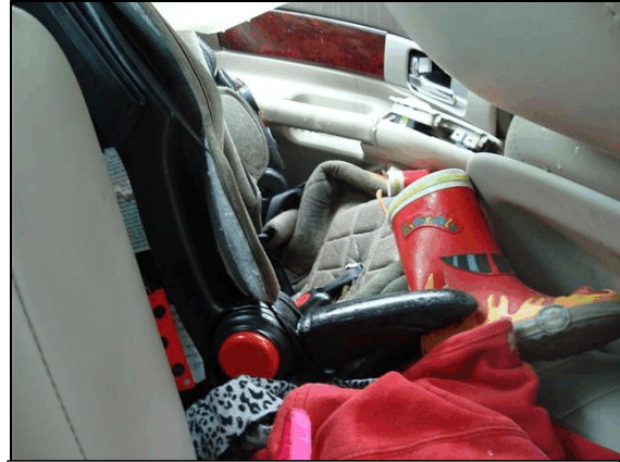
Figure 7. Second row left side door intruding into occupant compartment, 2004 Lincoln LS (police photo)
