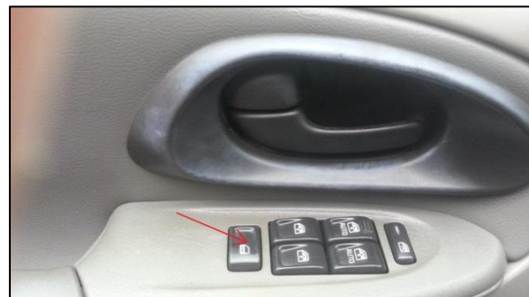
Figure 4. Exemplar vehicle driver's power door lock switch (arrow).
