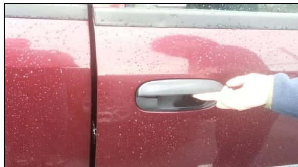
Figure 7. Exemplar vehicle exterior door handle in the open/unlatched position.
