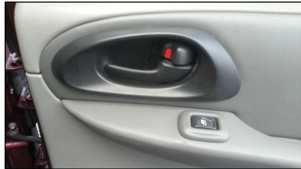
Figure 5. Unlocked position of the manual rotating lock lever of an exemplar vehicle.
