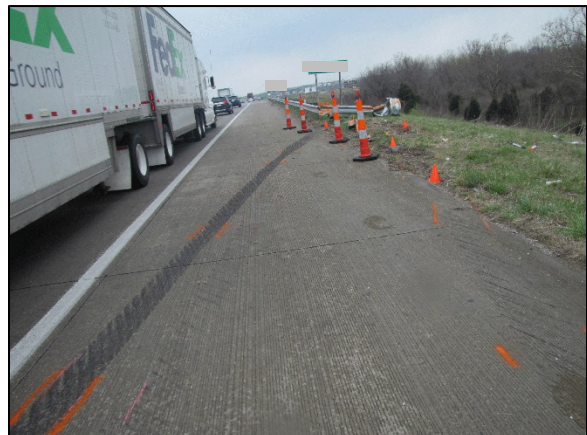
Figure 5: Path of travel of Chevrolet in clockwise yaw approaching impact with the end terminal, view west
