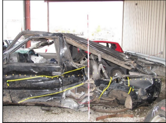
Figure 9: Area of guardrail kink penetration into second row
