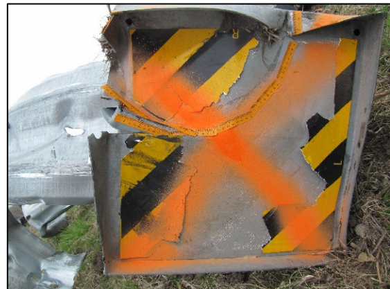
Figure 7: Shape of Chevrolet’s left front wheel rim stamped into face of end terminal
