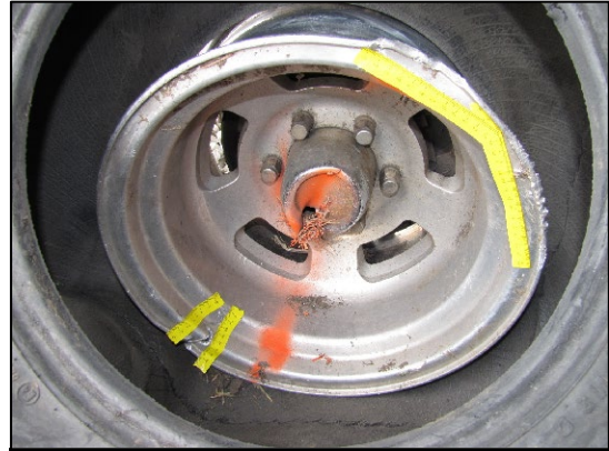
Figure 6: Damage to the Chevrolet’s left front wheel rim from the impact with the end terminal
