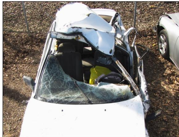
**Figure 14:** Overhead view of the Toyota with the separated roof repositioned for documentation purposes.
