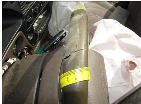
**Figure 17:** Damage to the steering wheel rim that resulted from contact with the guardrail as it penetrated into the Toyota's interior.
