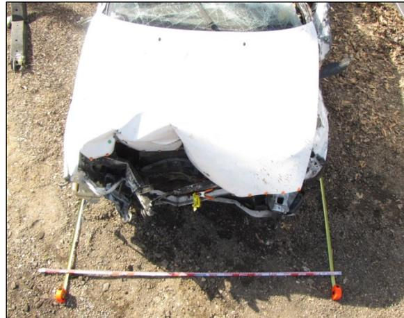
**Figure 12:** Overhead view of the Toyota depicting the frontal deformation.
