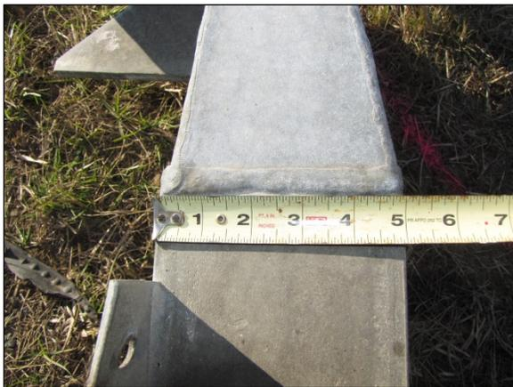
**Figure 7:** Measurement of the guide chute width of the ET-Plus end terminal device at the time of the SCI crash site inspection.
