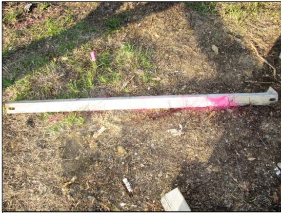
**Figure 9:** Displaced ground angle strut.
