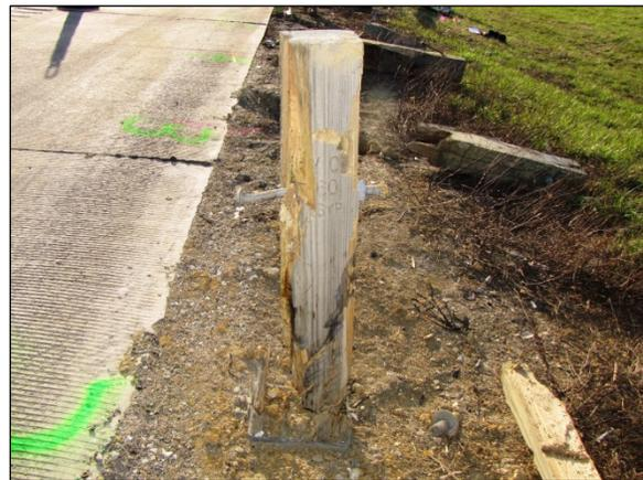
**Figure 8:** View of damaged Post 2 (repositioned for documentation during SCI reconstruction) and other sheared posts at the crash site.
