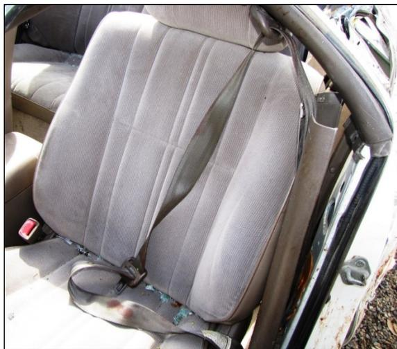
**Figure 20:** Toyota driver's lap and shoulder safety belt system at the time of the SCI vehicle inspection.
