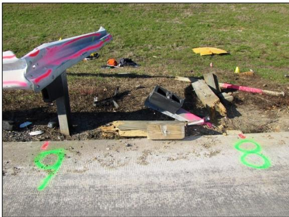
**Figure 10:** View of deformed Post 8 and Post 9 at the time of the SCI crash site inspection.
