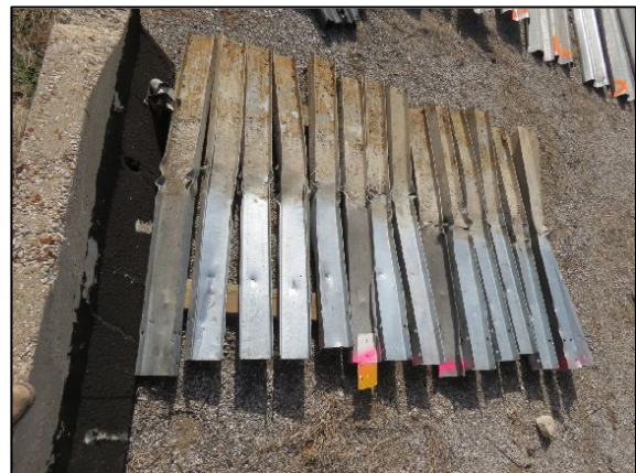
Figure 10: Remaining damaged posts
