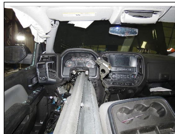
Figure 7: Path of guardrail penetration into the driver's seating position
