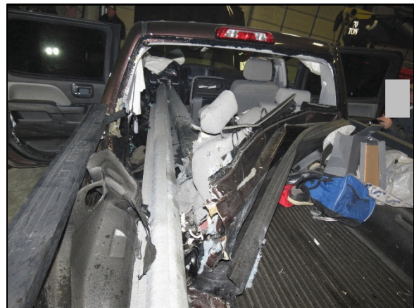
Figure 2: Back view of the guardrail penetration through the cab of the Chevrolet
