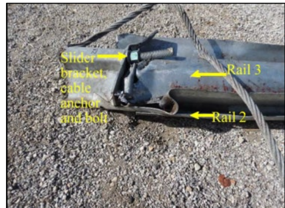
Figure 6: Rails 2, 3, and anchor cable bracket and bolt
