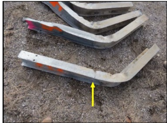
Figure 9: Post 3; arrow shows crimp in post remains closed
