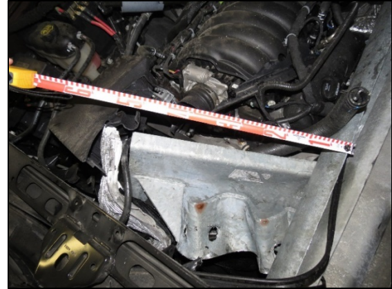
Figure 5: The end terminal entrapped in the Chevrolet's engine compartment, view from front left corner
