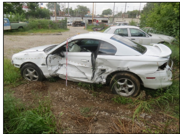
Figure 6: Damage to the left plane of the Ford from the impact with the deformed guardrail
