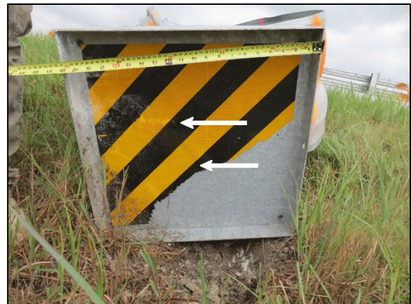
Figure 5: Area of contact to the face of the SKT from the impact with the Ford
