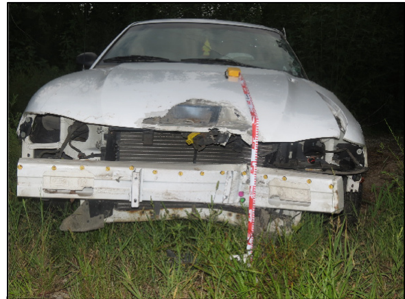
Figure 4: Damage to the Ford's front plane from the impact with the SKT
