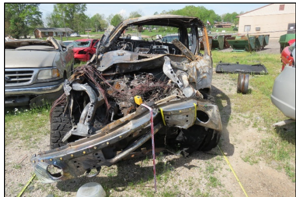
Figure 5: Damage to the front plane from the impact with the End terminal
