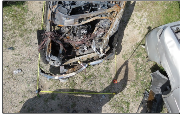
Figure 9: Top view of the crush to the front plane of the Ford
