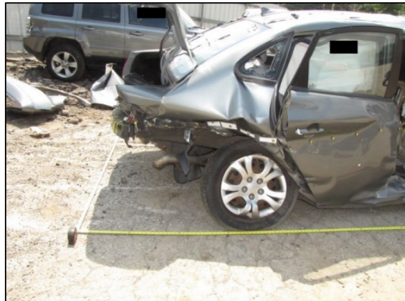
Figure 11: Right lateral image of the Hyundai depicting the Event 3 damage.
