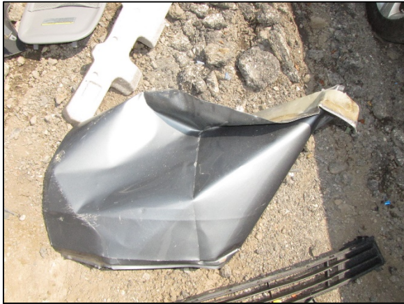
Figure 9: Direct contact damage on the right front door panel from the head of the SKT end treatment.
