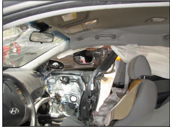
Figure 12: Lateral interior image of the Hyundai depicting the door intrusion
