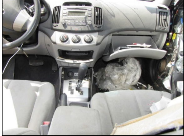
Figure 14: Console-mounted shifter deflected right from driver right thigh contact.
