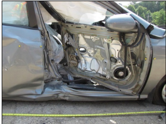
Figure 10: Deformation to the right front door of the Hyundai from the impact end terminal.
