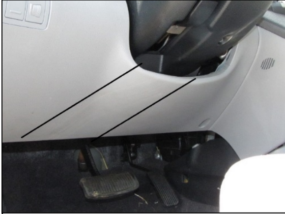
Figure 13: Left leg/foot scuff to the lower instrument panel/knee bolster.
