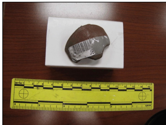
Figure 15. Inflator fragment found in vehicle, 2001 Honda Civic.
