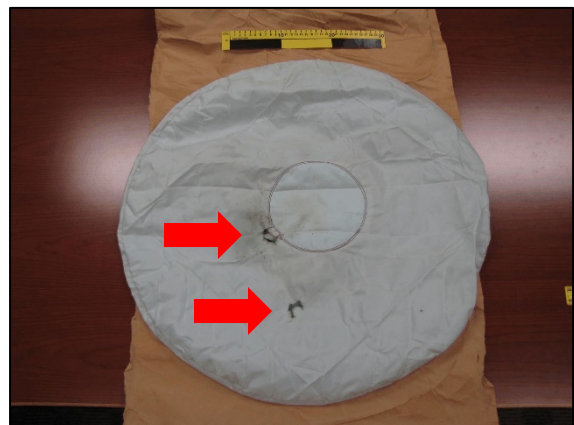
Figure 9. Holes in driver air bag front panel, 2001 Honda Civic.
