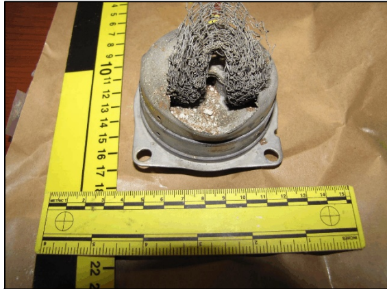
Figure 12. Ruptured inflator, 2001 Honda Civic.
