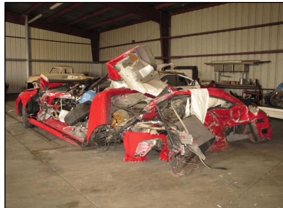
Figure 21. Back and left side damage, 2007 Toyota Solara.
