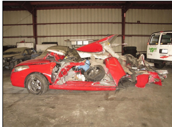
Figure 2. 2007 Toyota Solara, left side damage.
