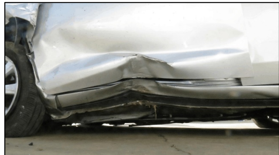
Figure 11. 2015 Toyota Yaris, left sill damage.
