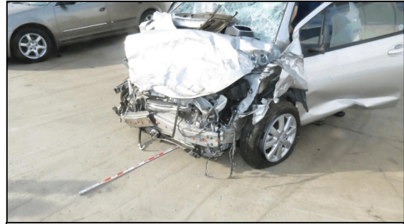
Figure 9. 2015 Toyota Yaris, frontal damage.
