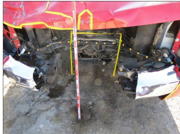
Figure 6: Damage to the front plane of the Chevrolet from impact with the end terminal
