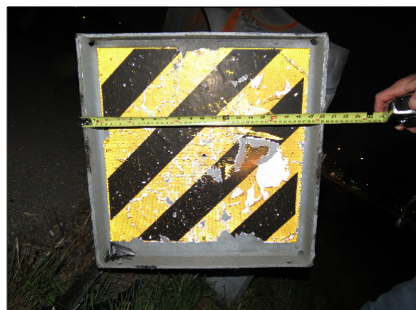
Figure 8: Minor damage to the face of the ET-2000
