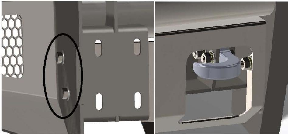
Figure 10a (bolt location for lower guard)
