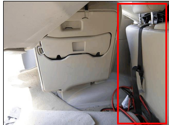
Figure 8: CRS tether strap to anchor connection, 2007 Lexus GX470 (police image).
