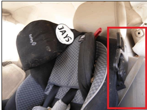
Figure 7: Lap and shoulder seat belt used to install Safety 1st CRS, 2007 Lexus GX470 (police image).
