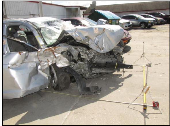
Figure 8: Right lateral view of the Honda at the front plane showing the extent of damage.
