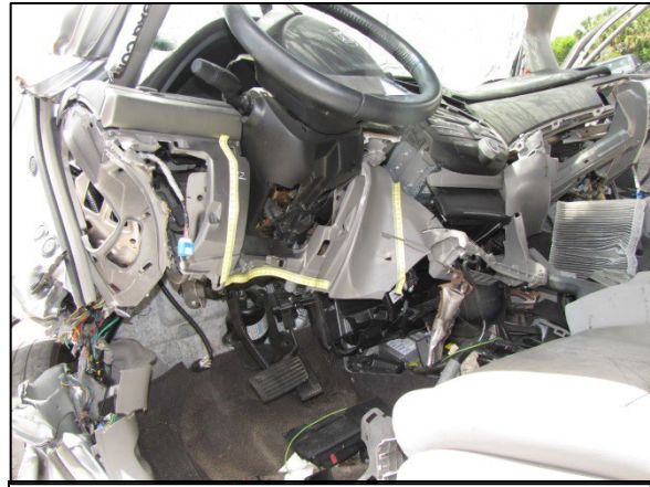
Figure 11: Oblique view of the driver's position in the Honda and the knee bolster contacts.
