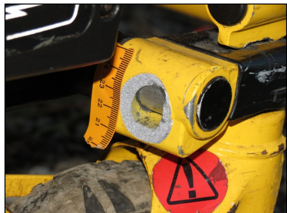
Figure 12: Fracture site on rear bracket of rail clamp securement bar.
