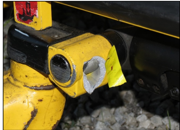
Figure 11: Fracture site on front bracket of rail clamp securement bar.
