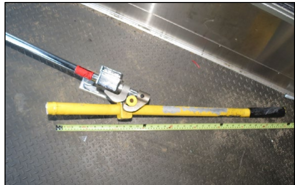
Figure 10: Cot's fractured rail clamp securement bar remained in rail clamp.
