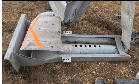
Figure 7: Extruded guardrail from the end terminal.
