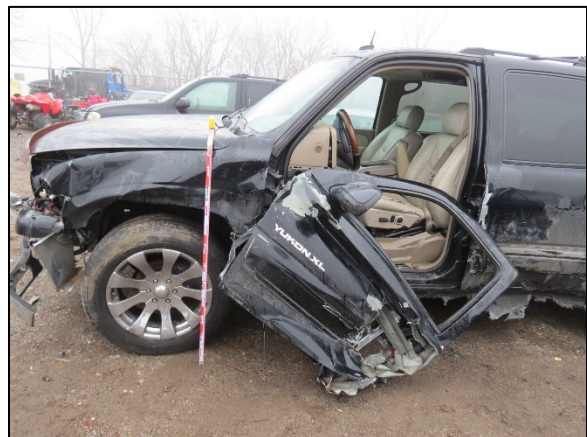
Figure 6: Damage to GMC's left front door from impact with kink in guardrail.
