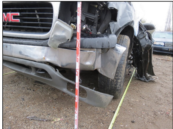
Figure 4: Damage to the front left corner of the GMC from impact with the ET-Plus.
