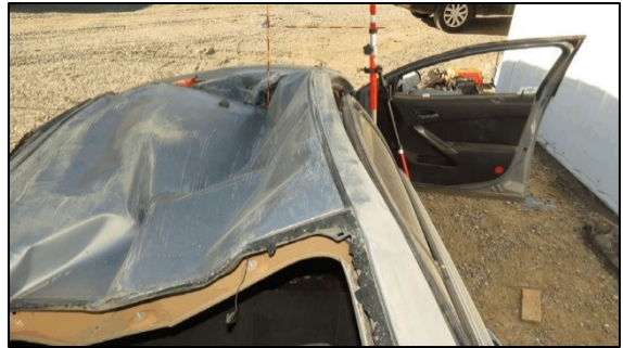
Figure 6. Rollover damage, 2009 Pontiac G6
