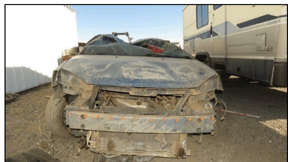
Figure 5. Frontal damage, 2009 Pontiac G6
