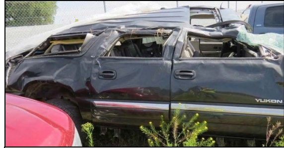
Figure 8. Right side intrusion, 2004 GMC Yukon
