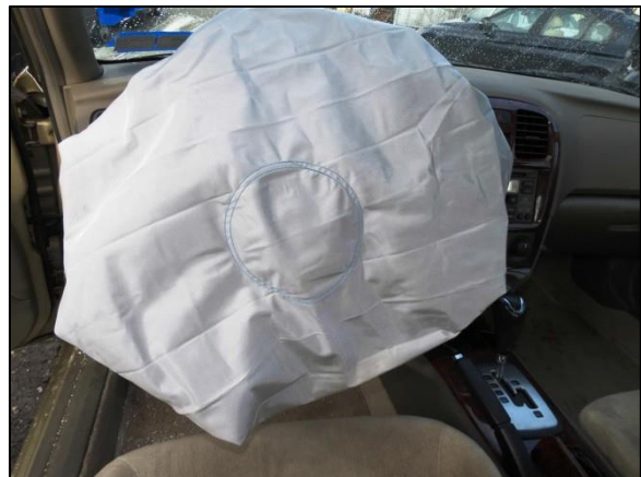
Figure 13: Interior image of the Hyundai showing the deployed driver air bag.
