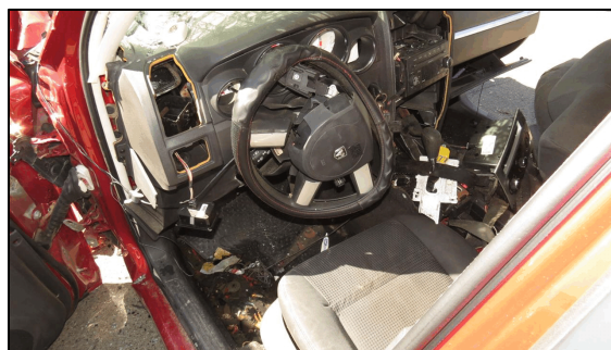
Figure 5. Steering wheel deformation, 2010 Dodge Charger
