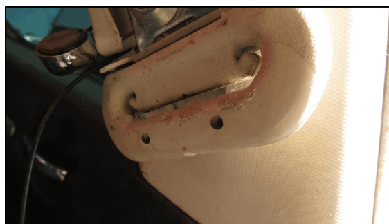
Figure 6. Upper anchor D-ring, 2010 Dodge Charger
