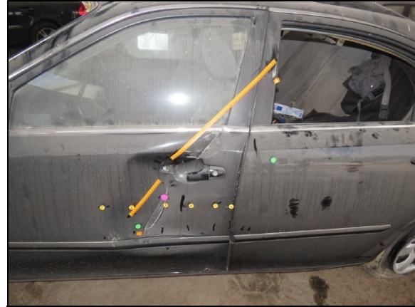
Figure 8: Left front door/B-pillar damage from guy wire impact
