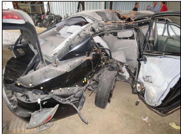
Figure 7: Right rear undercarriage/sill impact area.
