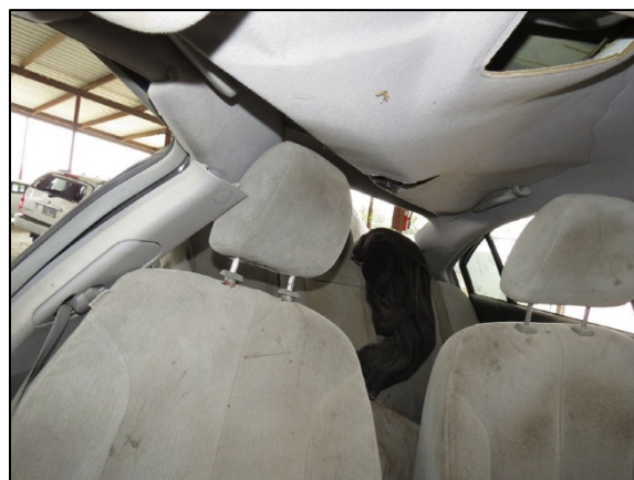
Figure 9: Right B-pillar intrusion
