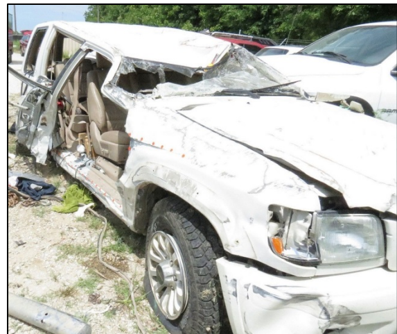
Figure 8. Right plane damage, 2001 Isuzu Trooper
