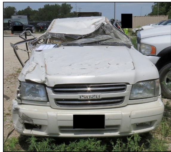
Figure 10. Rollover damage, 2001 Isuzu Trooper
