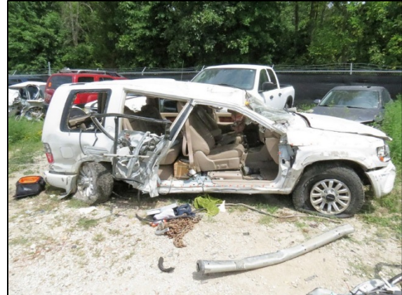
Figure 9. Right plane damage, 2001 Isuzu Trooper
