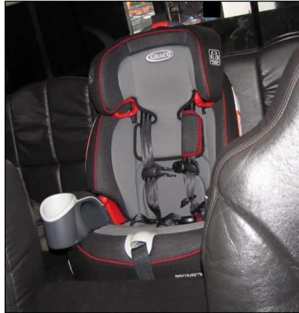
Figure 10: The CRS installed in the second row center position of the Dodge.
