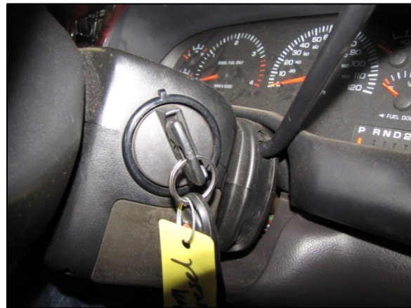
Figure 9: Keyed ignition switch of the Dodge in the lock position.
