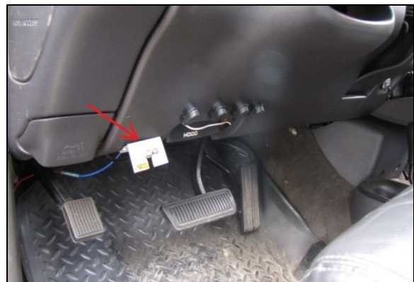
Figure 7: Aftermarket cable-pull fuel cut-off in the Dodge.
