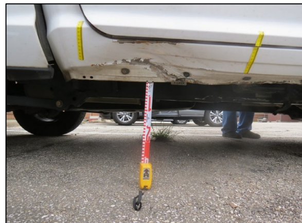
Figure 10. Undercarriage damage (right sill), 2014 Ram 1500.
