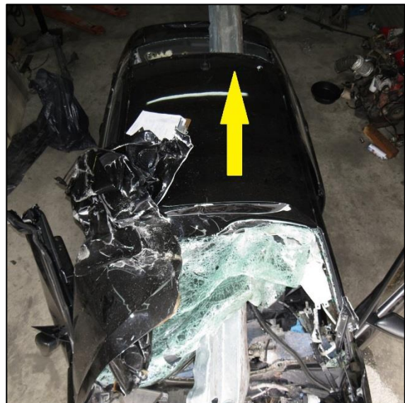
Figure 6. 2016 Volkswagen Jetta, guardrail panel intrusion. Arrow indicates guardrail exiting vehicle through backlight.
