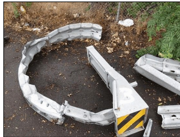
Figure 6. FLEAT end terminal and extruded W-beam.
