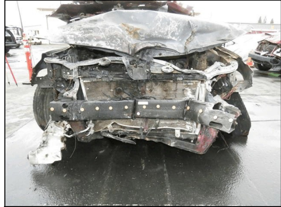
Figure 9. Front plane crush measurement, 2013 Toyota Avalon.
