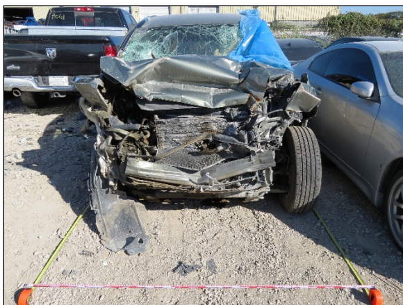
Figure 5. Frontal damage pattern and deformation to the 2007 Honda CR-V.
