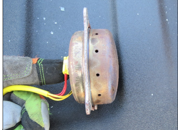
Figure 12. Lateral view of the Honda's air bag inflator, removed from the module during SCI documentation.
