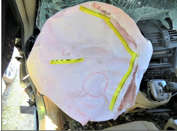
Figure 11. Deployed driver's frontal air bag with burst fabric, highlighted by yellow marking tape.
