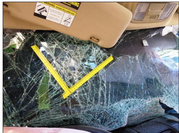
Figure 9. Contact to the windshield glazing from the Honda driver's head.
