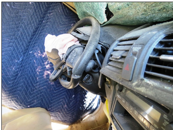
Figure 8. Steering wheel rim/column deformation in the Honda from driver loading.
