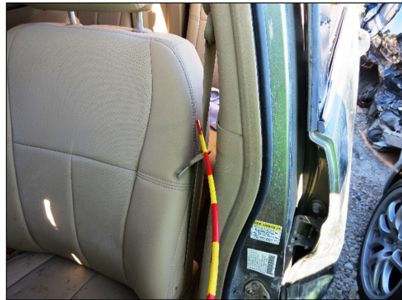
Figure 10. Driver's 3-point lap and shoulder seat belt system in the 2007 Honda CR-V.
