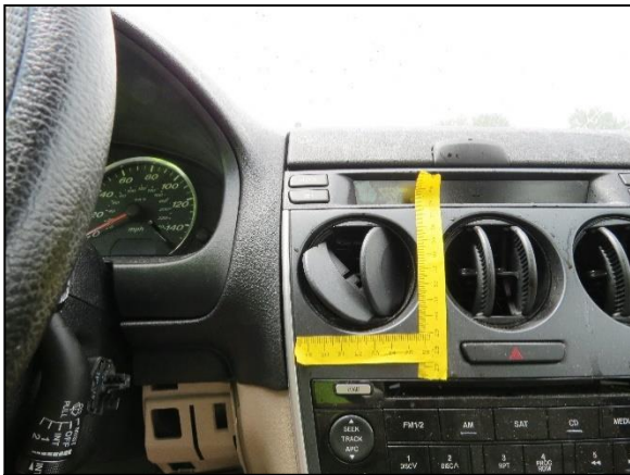
Figure 7: Fractured vent louvre in the Mazda.
