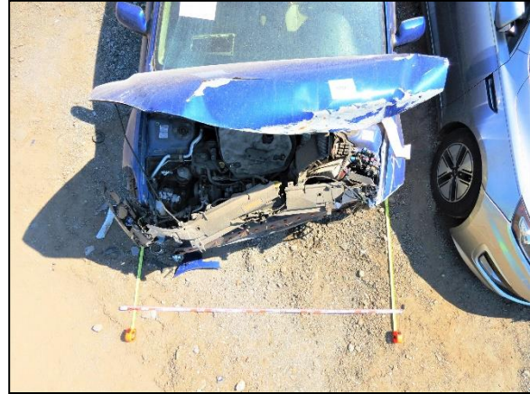
Figure 6: Overhead view of the front crush profile to the Mazda.
