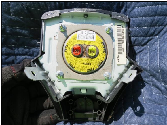
Figure 11: Driver’s frontal air bag module from the Mazda as found in the vehicle during the SCI inspection.
