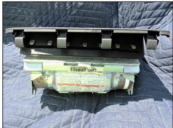
Figure 12: View of the Mazda’s passenger’s frontal air bag module at the time of the SCI inspection.
