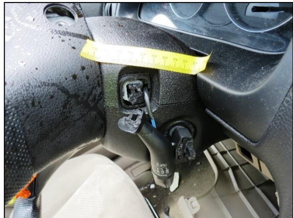
Figure 8: Fractured signal/wiper stalk in the Mazda.
