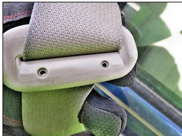
Figure 10: Latch plate of the Mazda's driver seat belt system with visible loading abrasions in the belt path.
