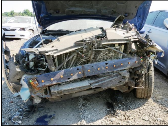
Figure 5: View of the front plane crush profile as documented during the SCI inspection.
