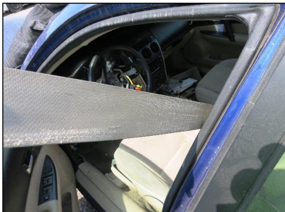
Figure 9: Webbing of the driver seat belt system in the Mazda with polymer transfer from the D-ring.
