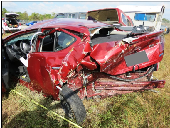
Figure 4: Rear plane damage to the 2009 Nissan Versa.
