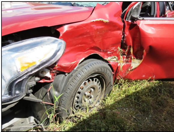
Figure 6: Event 2 impact damage to the left front corner area of the Nissan.
