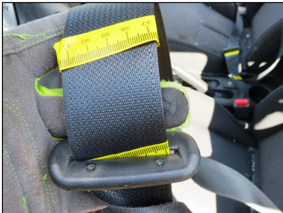
Figure 12: Loading evidence on the Nissan driver's 3-point lap and shoulder seat belt system.
