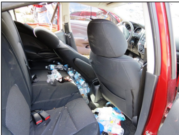
Figure 10: The Nissan's deformed front row seatbacks.
