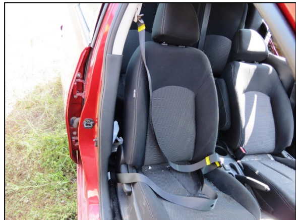
Figure 13: View of the Nissan's front right passenger's seat belt system with the occupant loading evidence identified.
