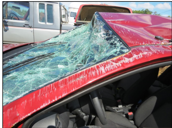
Figure 7: Vertical deformation to the Nissan's roof.
