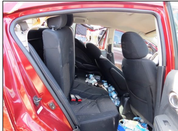
Figure 9: Forward displacement of the Nissan's second row seatback as viewed from the second row right position.
