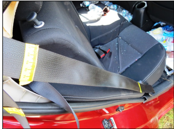
Figure 14: Loading evidence to the second row right seat belt system in the Nissan.
