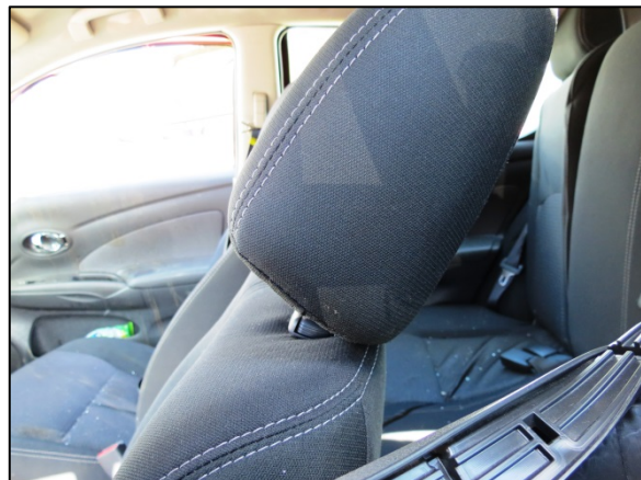
Figure 11: Nissan driver's deformed head restraint.
