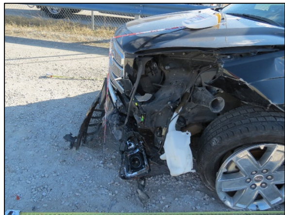
Figure 5: Left side view of the crush to the GMC’s bumper bar
