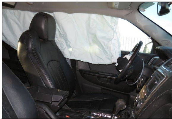
Figure 6: The GMC's deflated left IC air bag
