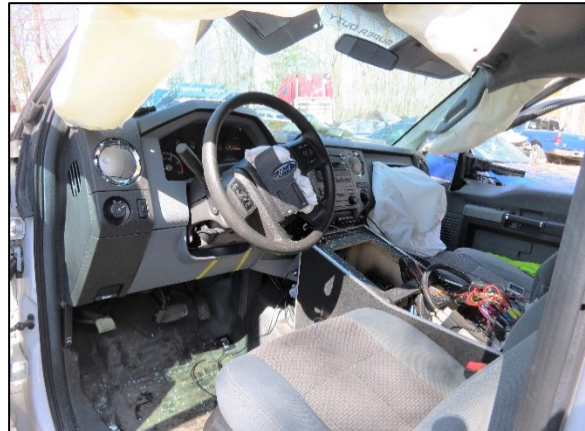
Figure 12: Crossing view of the ambulance cab interior, with the driver knee contact to the left lower instrument panel identified by yellow marking tape.
