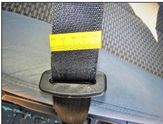
Figure 15: Latch plate loading transfer on the webbing of the Ford's driver safety belt system.
