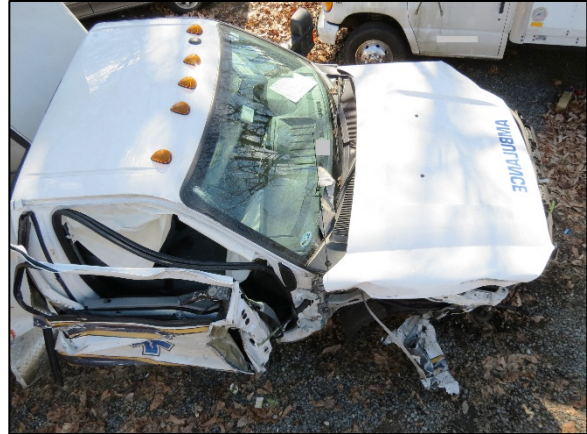
Figure 8: Right overhead perspective view of the ambulance cab and the magnitude of the damage extent.
