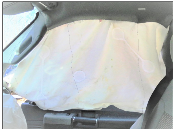
Figure 21: View of the deployed right IC air bag at the time of the SCI inspection.
