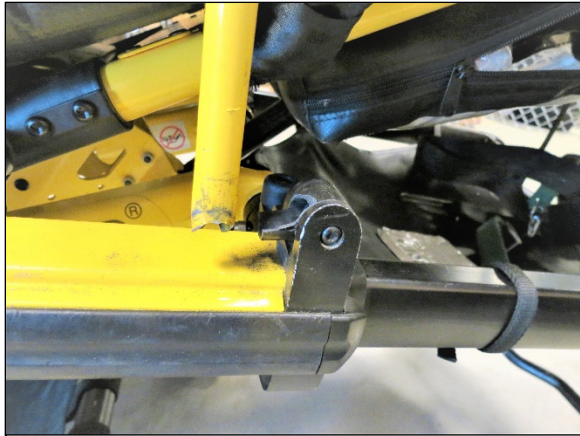
Figure 24: View of the fractured left arm rail support.
