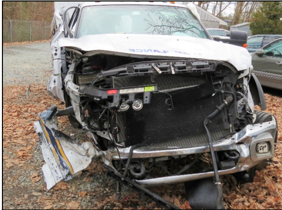
Figure 7: Front plane view of the 2016 Ford F-450 and its front plane damage profile.
