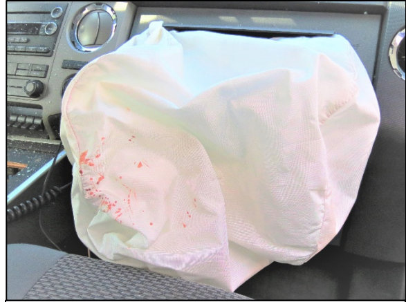
Figure 19: View of the deployed passenger's frontal air bag at the time of the SCI inspection.
