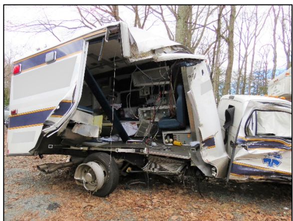
Figure 9: Right plane view of the Ford ambulance and the damage to the patient compartment.
