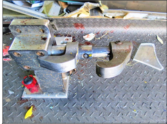
Figure 27: Disengaged locking clamp mechanism in the patient compartment.
