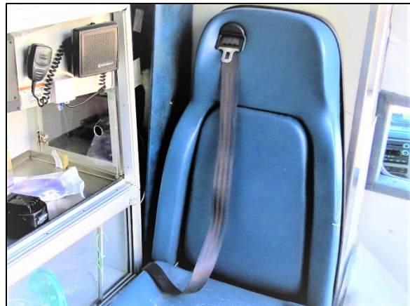
Figure 17: Three-point lap and shoulder safety belt system for the captain's chair position at the time of the SCI inspection.
