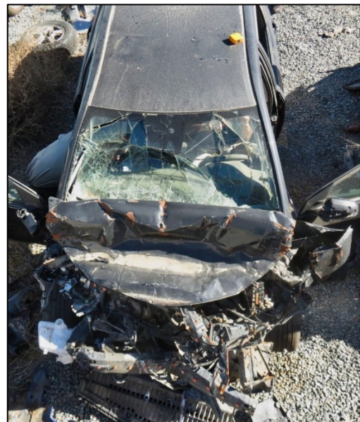
Figure 5. Frontal damage, 2018 Toyota Corolla.
