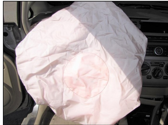
Figure 1. Deployed driver's frontal air bag, 2010 Nissan Versa.
