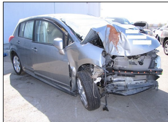
Figure 2. Front plane damage, 2010 Nissan Versa.
