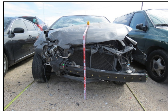
Figure 4: Front plane damage to the Corolla from impact with left plane of the Rav4.
